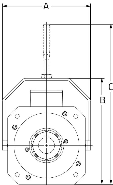
Optional Manual Release Handle works in either direction
