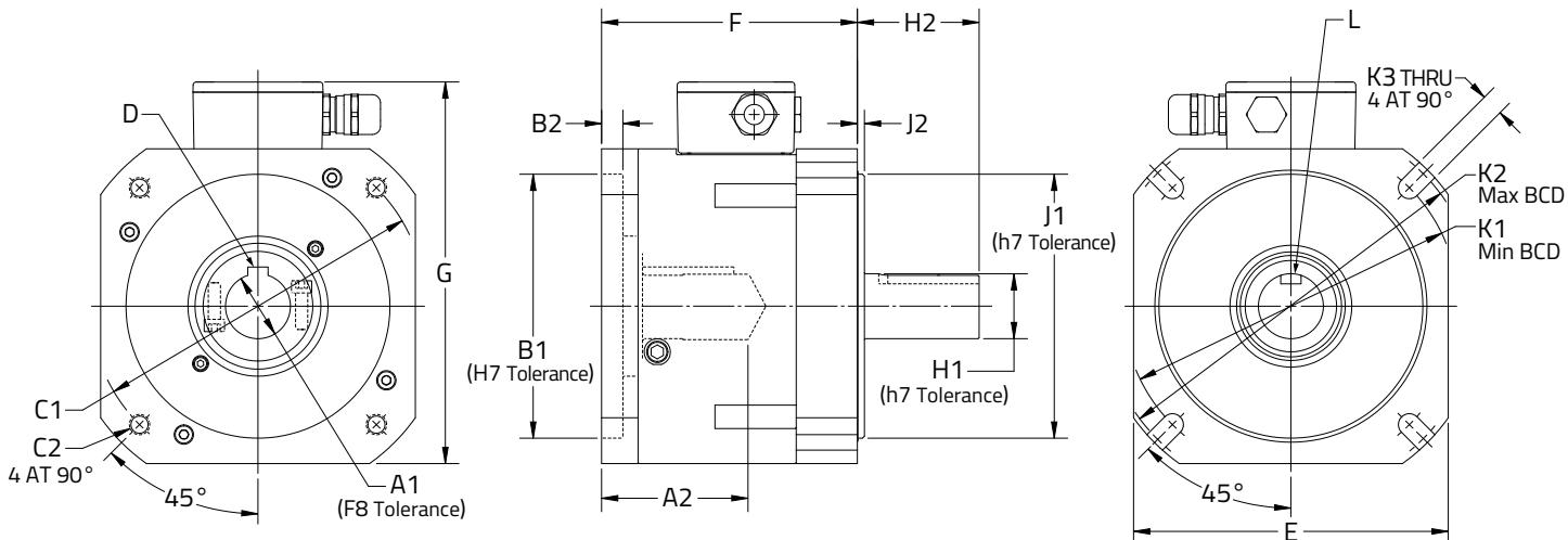
Contact Nexen to configure an Electric Servomotor Brake's dimensions for your application.
